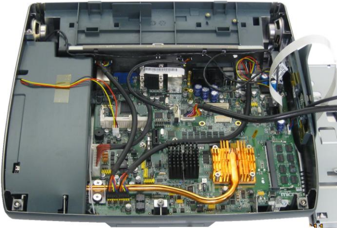
Internals of MICROS PCWS 2015, showing copper heat pipe leading from processor into cooling tunnel.
